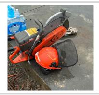
Power saw used for cutting rebar, had face shield and hearing protection provided.
