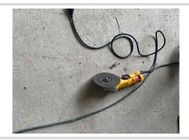
Another employee has a grinder that does not have its guard equipped. The employee complied to secure the guard.
