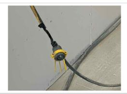
Sharp has a few cords that are damaged. Please ensure all cords are inspected and removed from service.
